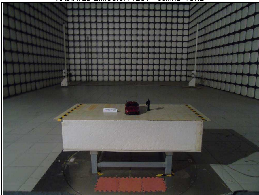
RADIATED EMISSION TEST < 30MHz~1GHz>
